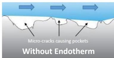
With the addition of **EndoTherm™** at the optimal concentration, the water hydrogen bonds are broken, thereby reducing the surface tension to as low as 27 mN/m, compared to 71 mN/m in untreated water. This alters the way steam bubbles form at the nucleated boiling sites along the imperfections found on the heating surfaces of fired boiler tubes.
