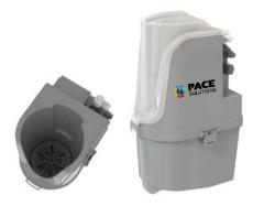
The **Dissolving Equipment** makes ready-to-be-fed product according to the demands of the water treatment program. Water is sprayed through a specially configured spray nozzle up into the bottle of concentrated treatment paste. The water dissolves a portion of the product and collects in in the reservoir. This liquified product is now ready to be fed into the water system.
