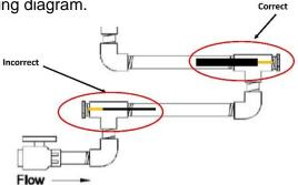
Due to the galvanic series of different metallurgy, the coupons must be installed in the following order when using multiple types of metal coupons:
